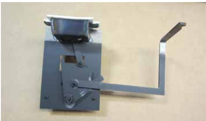
Figure 4.16 Timer Assembly with Gasket
