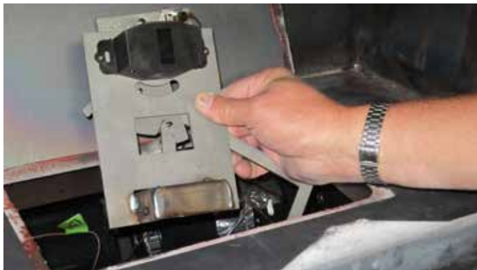
Figure 4.15 Removing Timer Assembly
