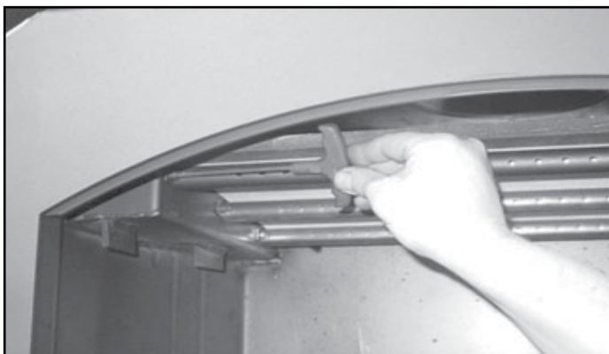
Figure 4.6 Removing Manifold Tube
