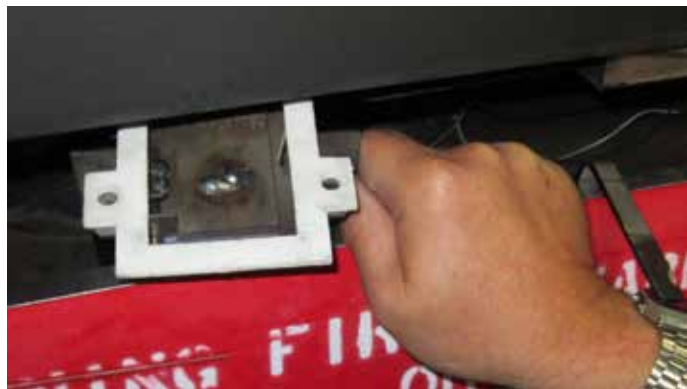
Figure 4.17 Inserting Timer Assembly With Gasket
