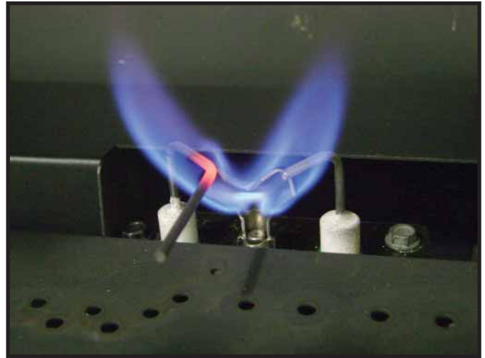
Figure 3.2 IPI Pilot Flame Patterns
