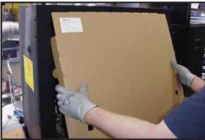
Figure 11.5 Installation of Splatter Guard
