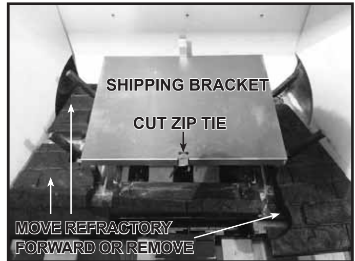
Figure 11.10 Separate Shipping Bracket from Log Grate
