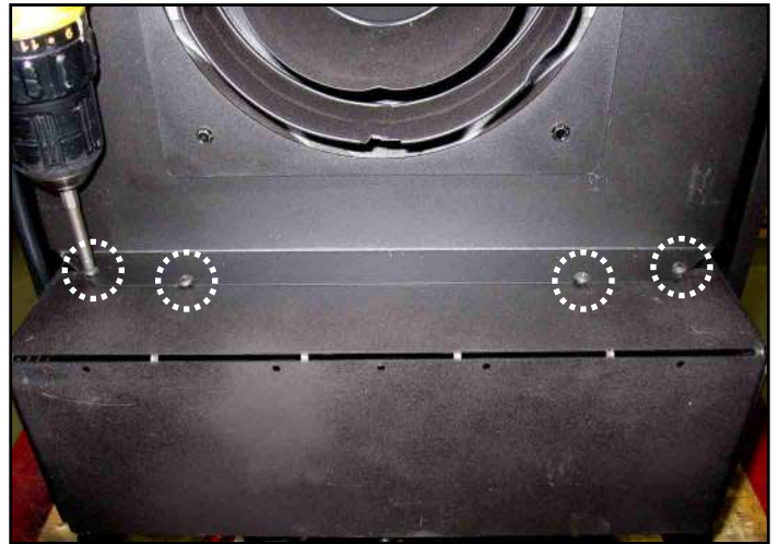
Figure 8.5 Attach Blower with Four Screws
