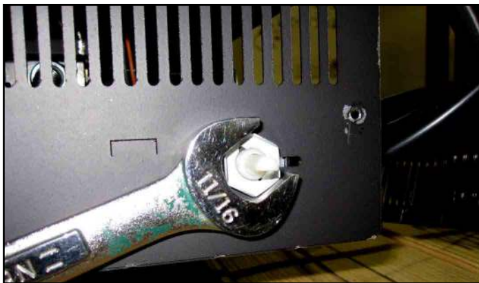
Figure 8.8 Mount Speed Control Using Pal Nut
