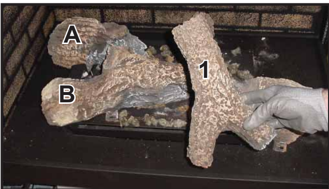
Figure 9. Placement of Log #1
