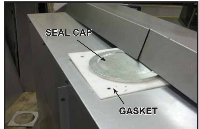
Figure 6.2 Seal Cap and Gasket Location
