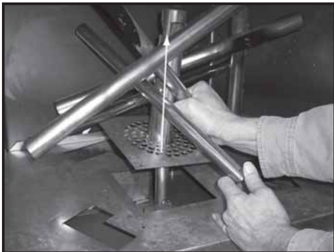
Figure 11.19 Remove Decorative Steel Log Assembly
