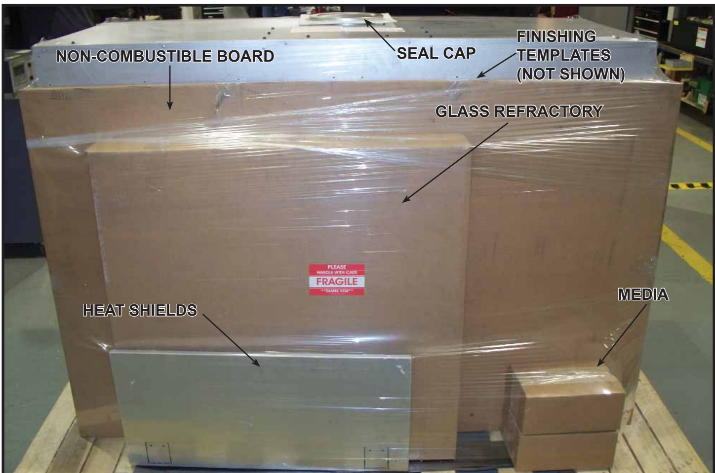
Figure 6.1 Shipping Location of Components
