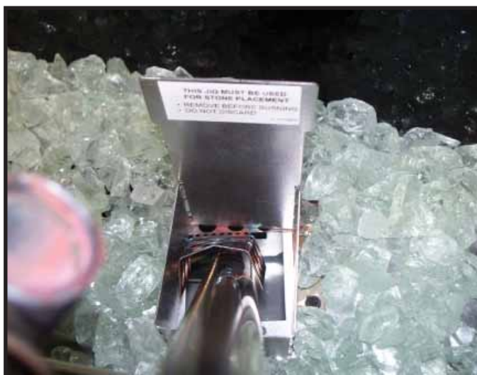
Figure 11.15 Remove Rock Media Jig
