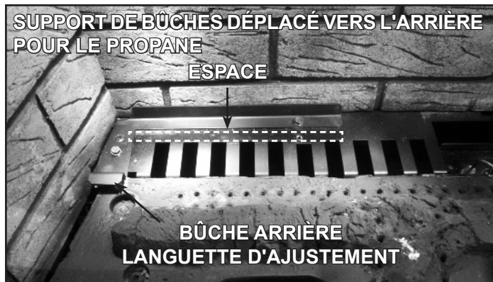
Figure 10.9 Position du support de bûches - propane
