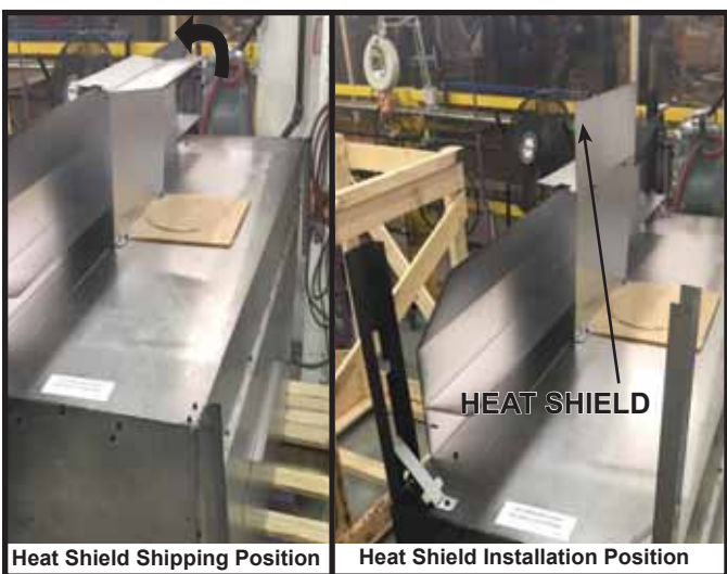
Figure 6.2 Heat Shield Shown Installed
