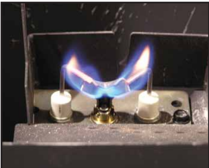
Figure 3.2 IPI Pilot Flame Patterns
