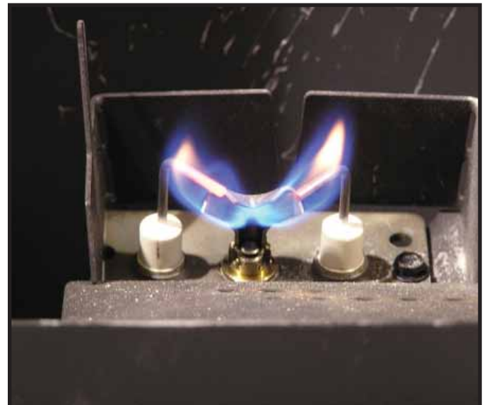
Figure 4.5 IPI Pilot Flame Patterns
