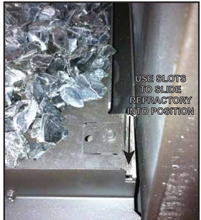
Figure 9.3 Install Refractory
