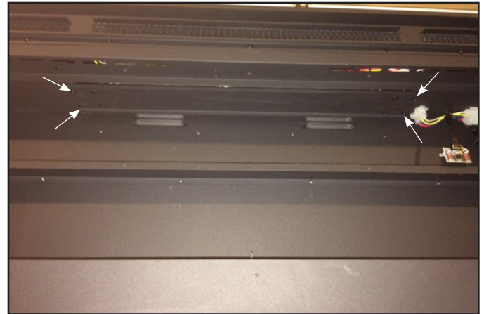
Figure 25. Remove Mounting Plate Screws
