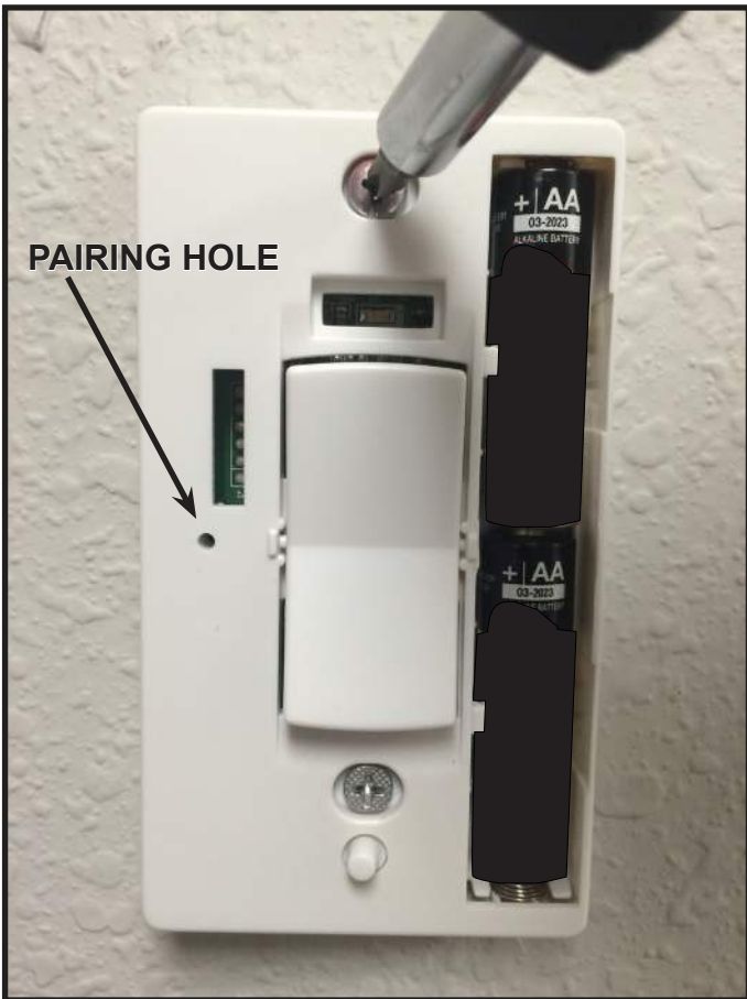
Figure 3. Mounting IFT-RC150 Wireless Wall Switch
