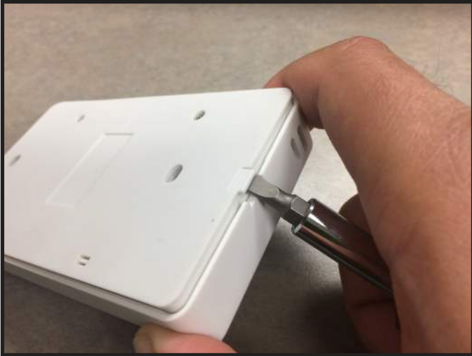
Figure 2. Wall Switch Disassembly
