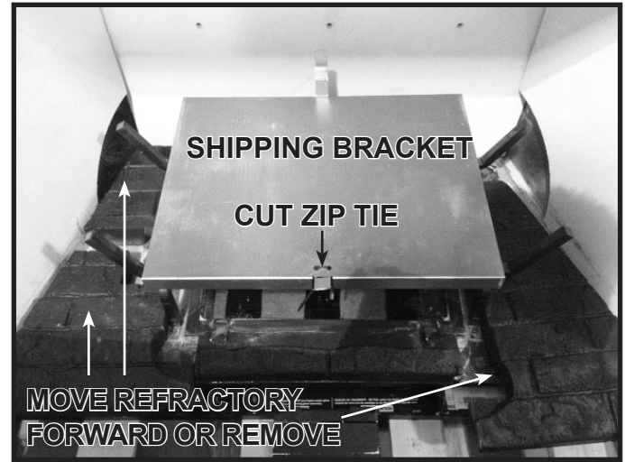
Figure 11.10 Separate Shipping Bracket from Log Grate
