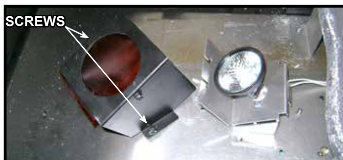
Figure 11.13 Light Housing Removed, Bulb Installed
