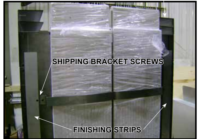
Figure 6.3 Shipping Brackets and Finishing Strip Locations.
