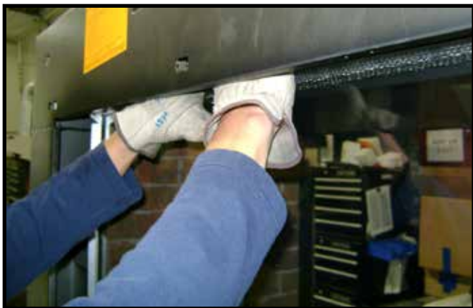
Figure 11.6 Top Glass Latch Access
