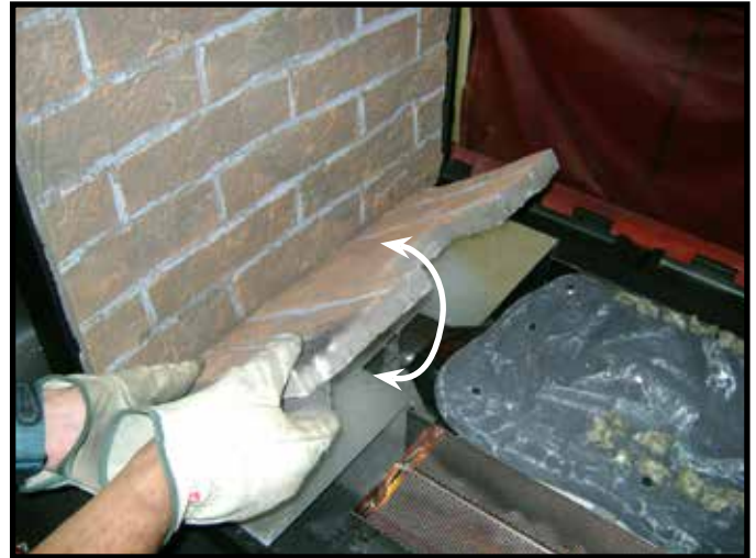
Figure 11.17 Positioning Inner Bottom Refractory
