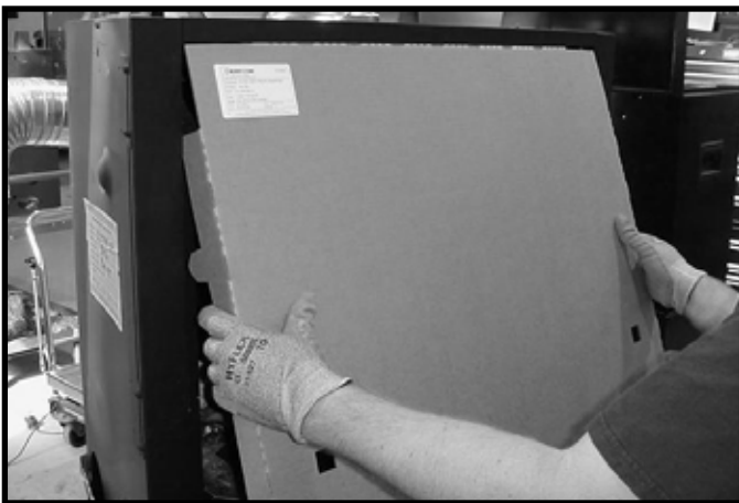
Figure 11.5 Installation of Splatter Guard
