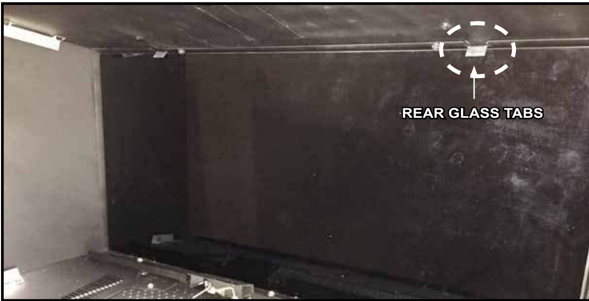
Figure 5 Install Rear Glass Panel
