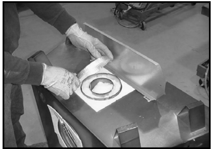
Figure 6.8 Remove the seal cap.
