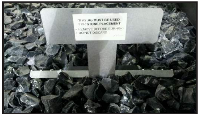
Figure 9.9 Rock Placement Jig
