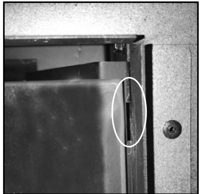
Figure 11.25 Slot for Barrier Glass Retaining Clip (Right Side Shown)
