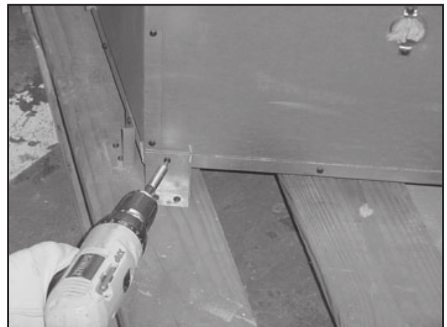
Figure 3.12 Removing Shipping Brackets
