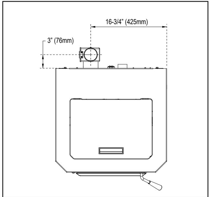
**Figure 10.3** - Top View w/ Top Vent Adapter (TPVNT-6)
