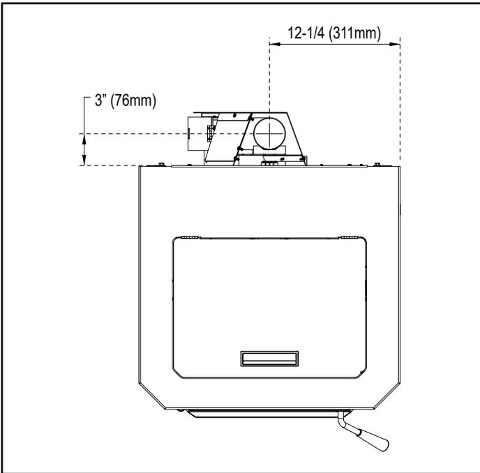
Figure 9.1 - Top View w/ Top Vent Adapter (TPVNT-7)
