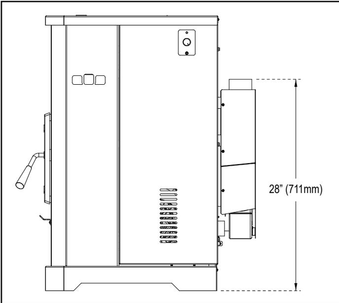
Figure 9.2 - Side View w/ Top Vent Adapter (TPVNT-7)
