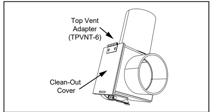
Figure 22.3 - 90° Rear to Top Vent Adapter (TPVNT-6)
