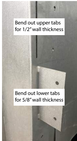
Figure 6.4 Nailing tab bent out for installation
